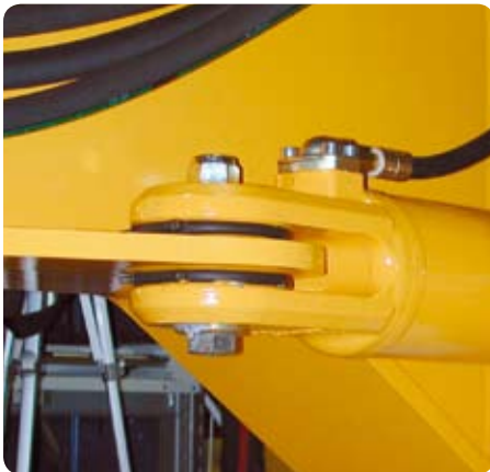
CARB in the steering cylinder rod end
